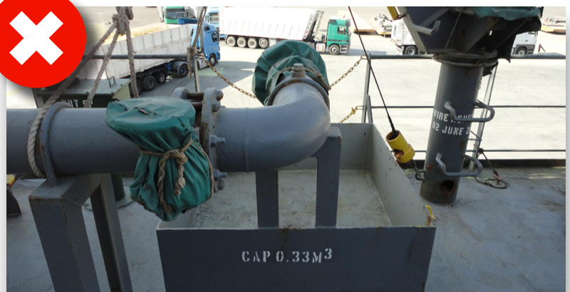
The test date, pressure and the medium used for the test should be also stenciled
